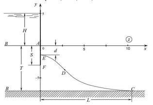
Fig. 1, 6. The current picture calculated at  $\varepsilon = 0.6$ , T = 7, S = 3, H = 7,  $H_0 = 3$  ux<sub>C</sub> = 100
