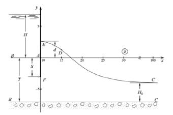
Fig. 1. a. The current picture calculated at  $\varepsilon = 0.6$ ,  $h_c = 0.5$ , T = 7, S = 3, H = 5.
