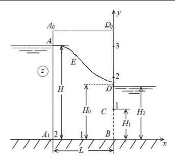
Fig. 2. The current picture in a rectangular jumper calculated at  $\epsilon = 0.5$ , H = 3, L = 2,  $H_1 = 1$ ,  $H_2 = 1.4$
