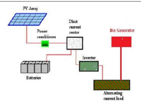
Figure 4. Hybrid PV-Biogas generator diagram for isolated site
