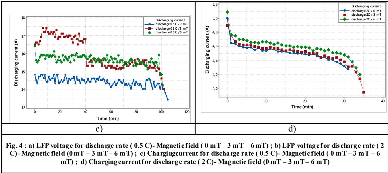
Fig. 4 : a) LFP voltage for discharge rate ( 0.5 C)- Magnetic field ( 0 mT – 3 mT – 6 mT) ; b) LFP voltage for discharge rate ( 2 C)- Magnetic field ( 0 mT – 3 mT – 6 mT) ; c) Charging current for discharge rate ( 0.5 C)- Magnetic field ( 0 mT – 3 mT – 6 mT) ; d) Charging current for discharge rate ( 2 C)- Magnetic field ( 0 mT – 3 mT – 6 mT)
