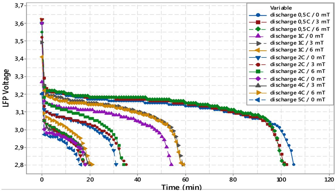
Fig. 9. LFP voltage for discharge rate ( 0.5 C – 1 C – 2 C – 4 C – 5 C)- Magnetic field ( 0 mT – 3 mT – 6 mT)
