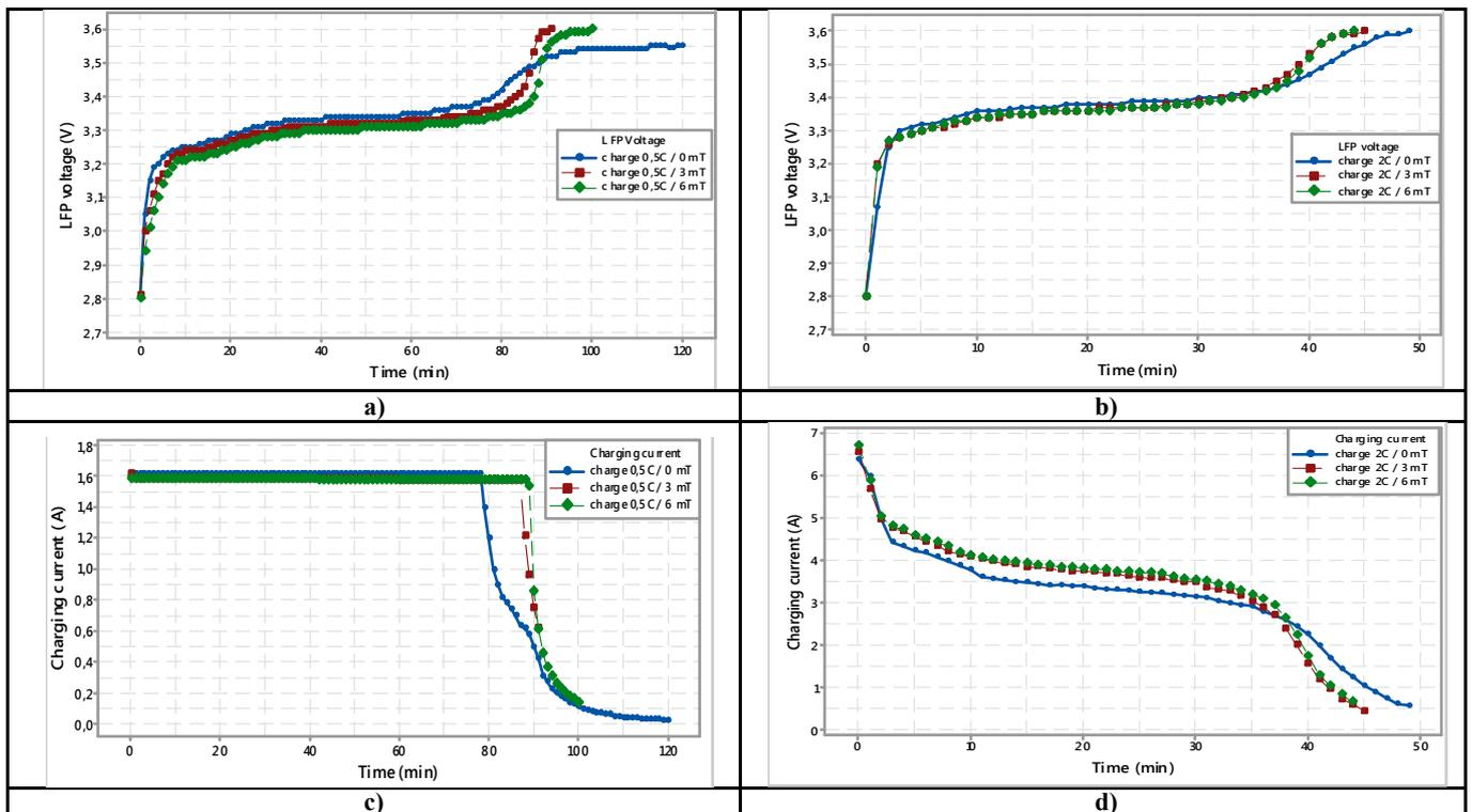
Fig. 7 : a) LFP voltage for charge rate ( 0.5 C) - Magnetic field ( 0 mT – 3 mT – 6 mT) ; b) LFP voltage for charge rate ( 2 C) - Magnetic field ( 0 mT – 3 mT – 6 mT) ; c) Charging current for charge rate ( 0.5 C) - Magnetic field ( 0 mT – 3 mT – 6 mT) ; d) Charging current for charge rate ( 2 C) - Magnetic field ( 0 mT – 3 mT – 6 mT)
