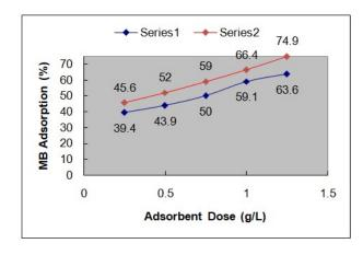
Series 1. KOH treated AC and Series 2: phosphoric acid treated AC
