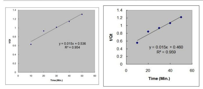
Figure 7. Fit of pseudo second order kinetics for MB dye adsorption on both (A) phosphoric acid and (B) KOH based activated carbon
