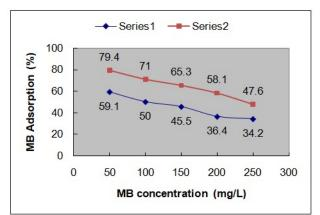
Series 1. KOH treated AC and Series 2: phosphoric acid treated AC
