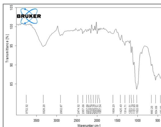
Figure 3. FTIR spectra of nanocellulose extracted from sugarcane bagasse
