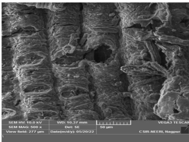
**Figure 4.** SEM images of nano cellulose extracted from sugarcane bagasse
