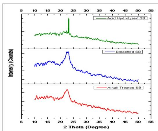
Figure 2. XRD graphs for alkali treated SB, bleached SB and acid hydrolysed SCB
