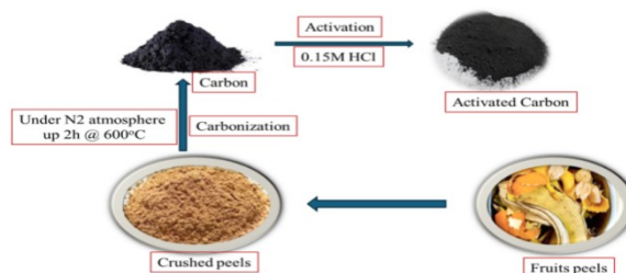
Figure 6. Preparation mechanism of activated carbon from fruit peels
