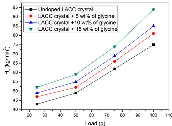
**Fig.7. Variation of microhardness number ( $H_v$ ) with the load for undoped and glycine doped LACC crystals**
