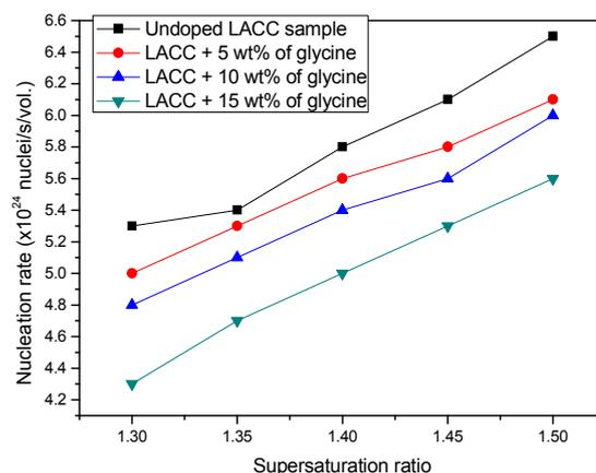
Fig.6. Plots of nucleation rate with supersaturation ratio for glycine doped LACC samples
