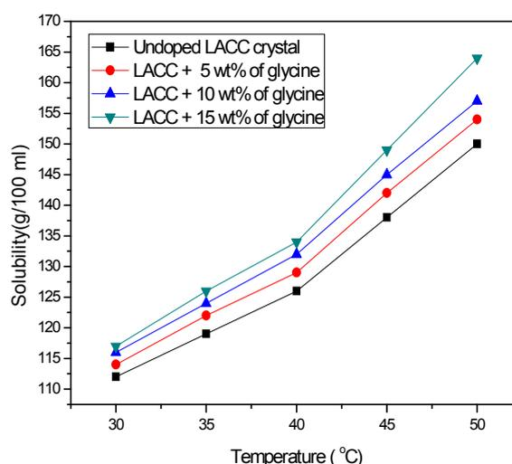
Fig.1. Solubility curves of undoped and glycine doped L-alanine cadmium chloride (LACC) samples
