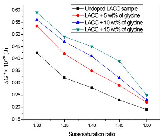
Fig.3. Plots of Gibbs free energy change with supersaturation ratio for glycine doped LACC samples
