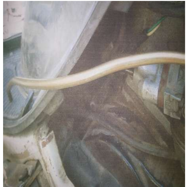
Figure 3. Copper Piping to Carburetor
