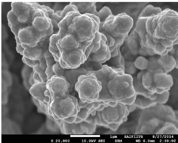
Fig. 4. SEM image of a typical tip of branch of copper dendrite
