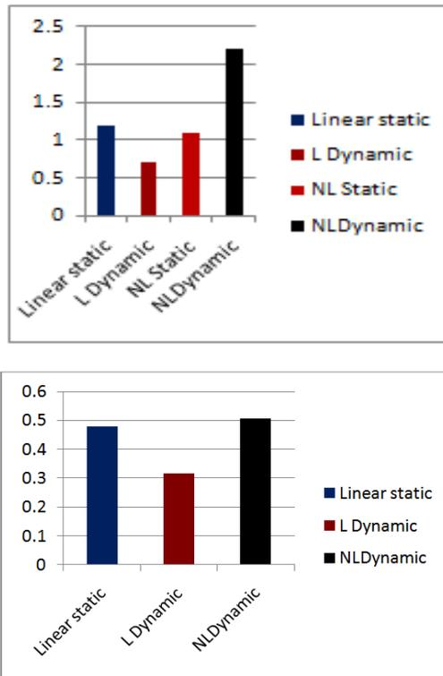
Fig.6. Demand-Capacity ratio and Roof displacement for column of transverse direction remove
