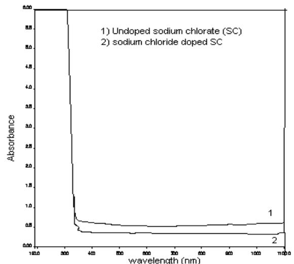
Figure 8. UV-visible absorbance spectra of f (a) pure and (b) NaCl doped  $\text{NaClO}_3$  crystals
