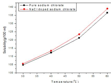
Figure 1. Solubility curves for pure and NaCl doped  $\text{NaClO}_3$  samples
