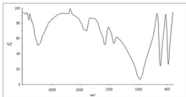
(ii) Pure NaClO<sub>3</sub>Figure 4. FTIR spectra of (i) NaCl doped NaClO<sub>3</sub> and (ii) pure NaClO<sub>3</sub> crystalsTable 4 (a). FTIR assignments for pure NaClO<sub>3</sub> single crystals
