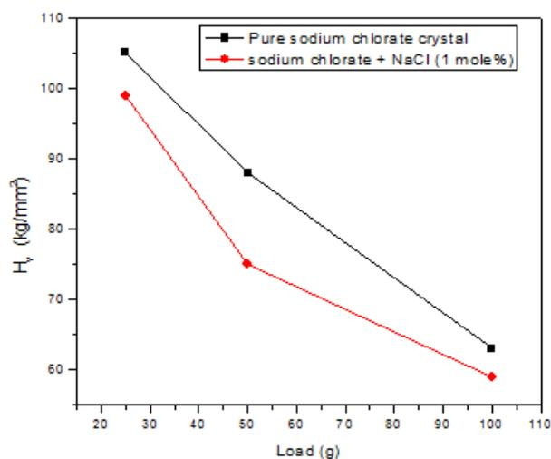
Figure 6. A plots of load P against hardness number (H<sub>v</sub>) for pure and NaCl doped NaClO<sub>3</sub> crystals
