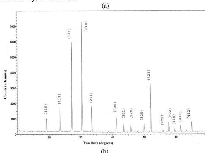
Figure 3. XRD patterns of (a) pure NaClO<sub>3</sub> and (b) NaCl doped NaClO<sub>3</sub> samples
