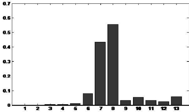
Fig: 3(b): Sine wave with voltage sag and its energy distribution diagram
