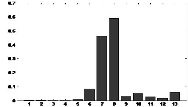
Fig: 3(c): Sine wave with voltage swell and its energy distribution diagram
