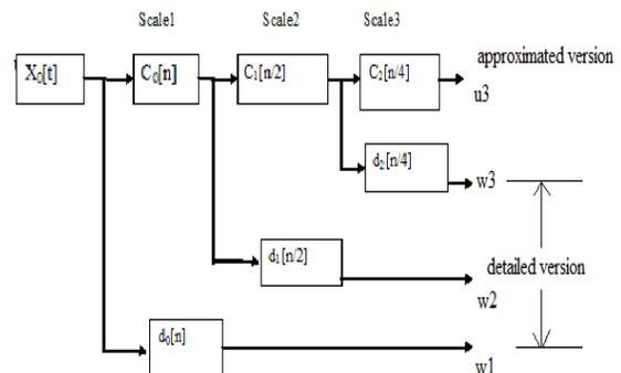
Figure 2. Three decomposition level of DWT
