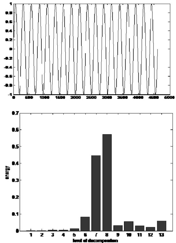
**Fig: 3(a) Pure sine and its energy distribution diagram**
