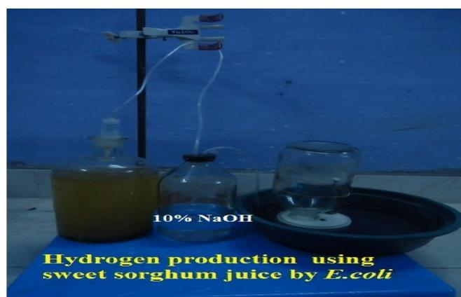
Figure 1. Collection of Hydrogen using water displacement method
