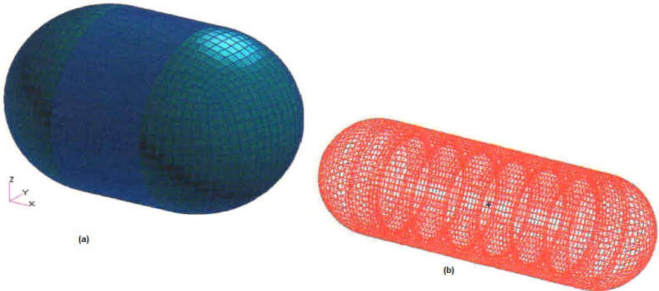
Fig. 4. Finite element modeling (a) fluid domain and explosion and (b) submersible hull
