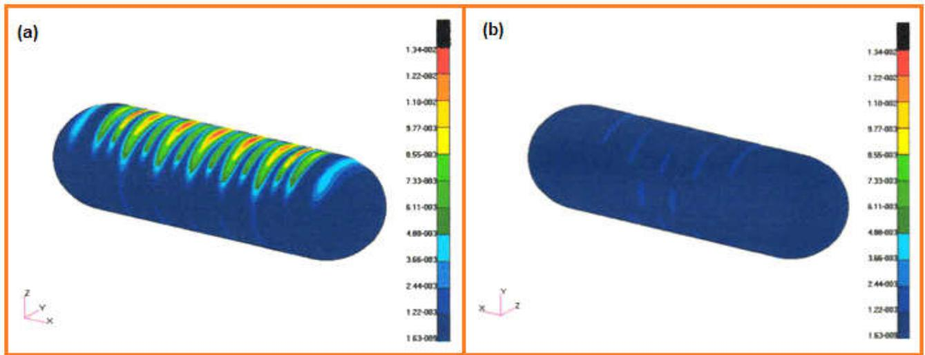
Fig. 8. Effective plastic strain of submerged hull at SF = 0.45 (a) surface exposed to explosion and (b) surface on the rear side of submersible hull
