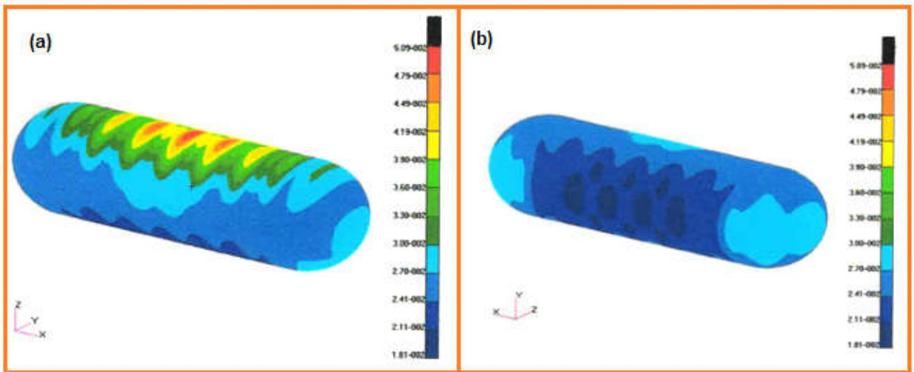
Fig. 6. Displacement of submerged hull at HSF = 0.45 (a) surface exposed to explosion and (b) Surface on the rear side of submersible hull
