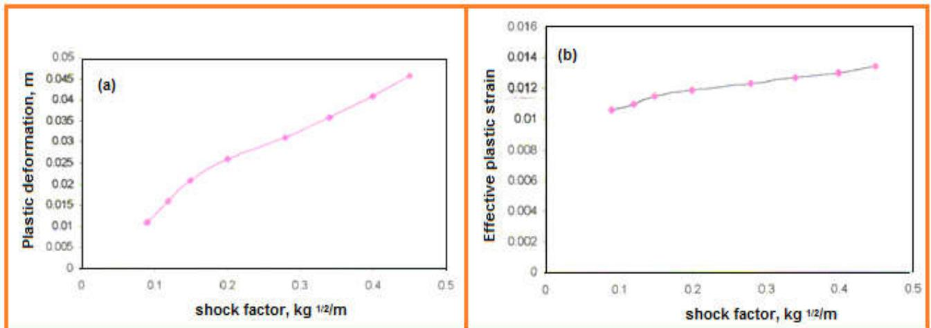
Fig. 9. Impact of shock load deflection (a) deformation (b) plastic strain
