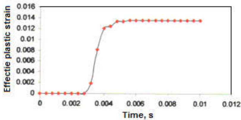
Fig. 7. Strain-time history for charge weight of 25 kg
