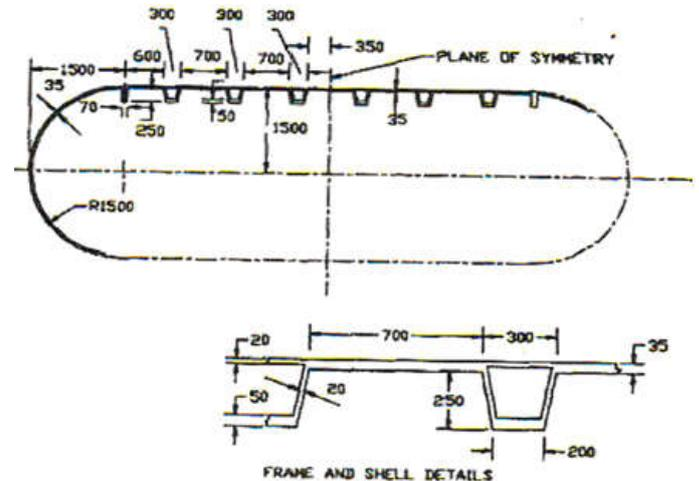
Fig. 3. Physical model of submersible hull
