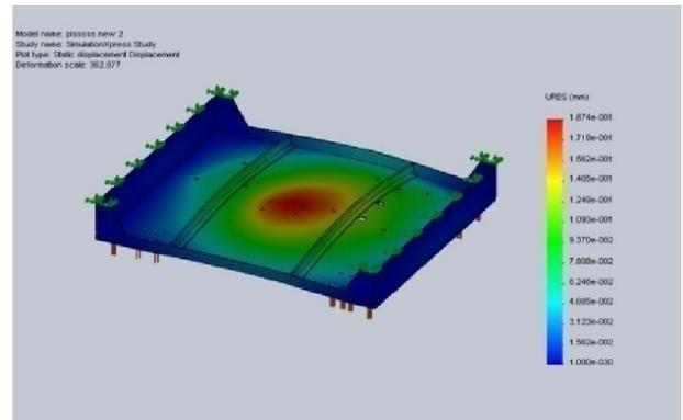
Fig. 7. Deformation of Base with 2 Ribs
