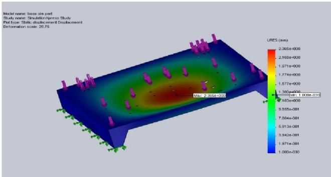
Fig. 3. Static deformation of base
