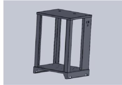
**Fig. 2. Assembled View Of Canopy**
