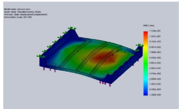
Fig 8. Deformation of base with 3 ribs
