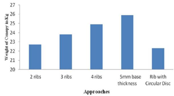
Fig. 12. Alternative Approaches vs Weight of canopy
