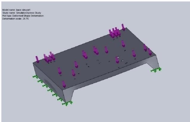
Fig. 5. Deformation shape of base
