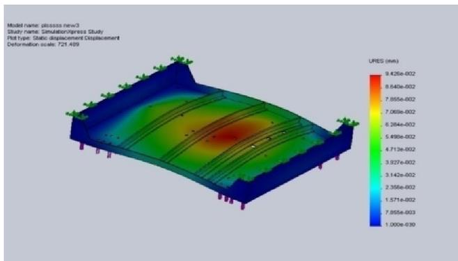
Fig. 9. Deformation of base with 4 ribs
