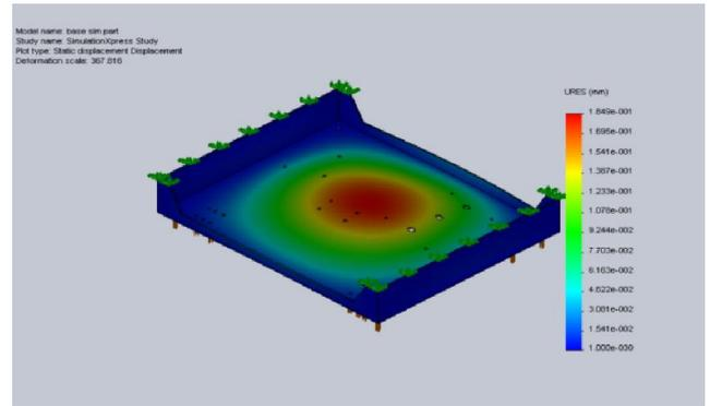
Fig. 6. Deformation of base with 5mm thickness
