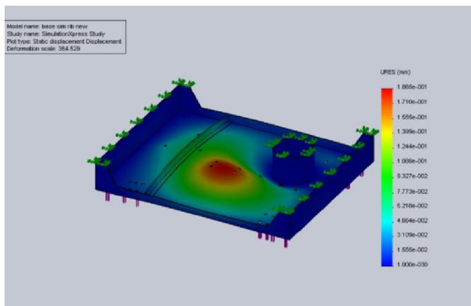
Fig 10. Deformation of base with circular structure
