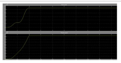
Figure 5(a). Active And Reactive Power at bus 1
