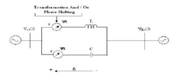
Figure 1. Operating Principle of IPC
