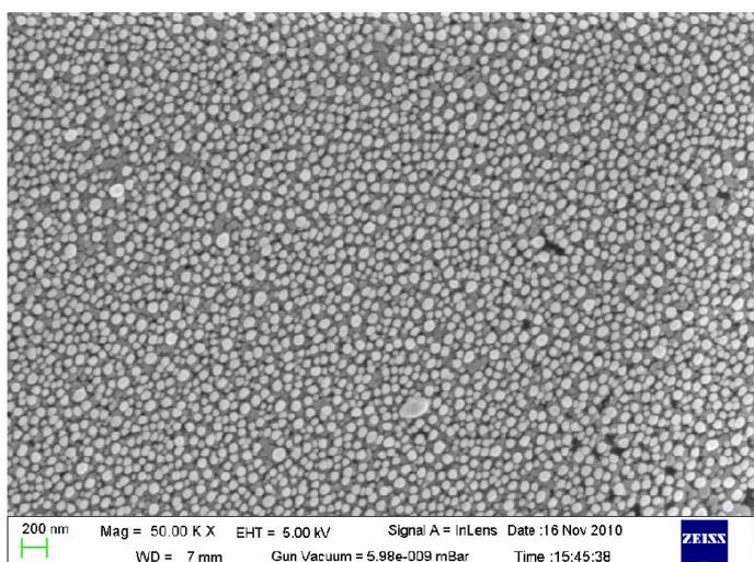
Fig. 2. FESEM images of the top view of ZnO nanorods grown by MOCVD using a two-step growth technique on fused quartz substrates
