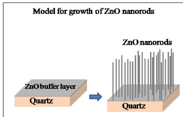
Fig. 3. (a) A graph showing the variation of growth temperature and growth duration for the formation of nanorods, (b) A model for the growth of ZnO nanorods
