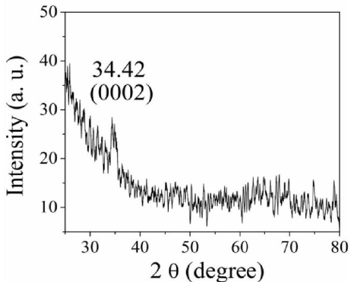
Fig. 1. X-ray diffraction pattern of ZnO nanorods grown by MOCVD using a two-step growth technique on fused quartz substrates
