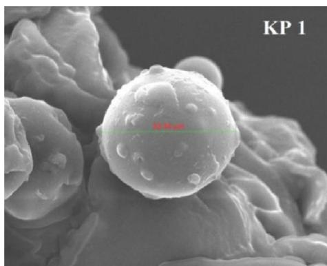
Fig. 5. SEM photographs of Lansoprazole microspheres
