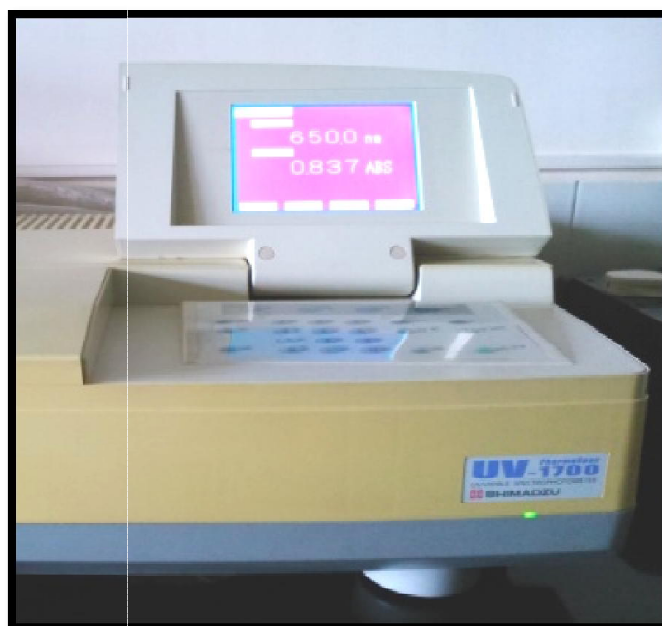
Fig. 3. Spectrophotometer Shimadzu UV 1700 giving the reading of optical density of stain remaining after completion of AB staining procedure as 0.837 at 650 nm wavelength
