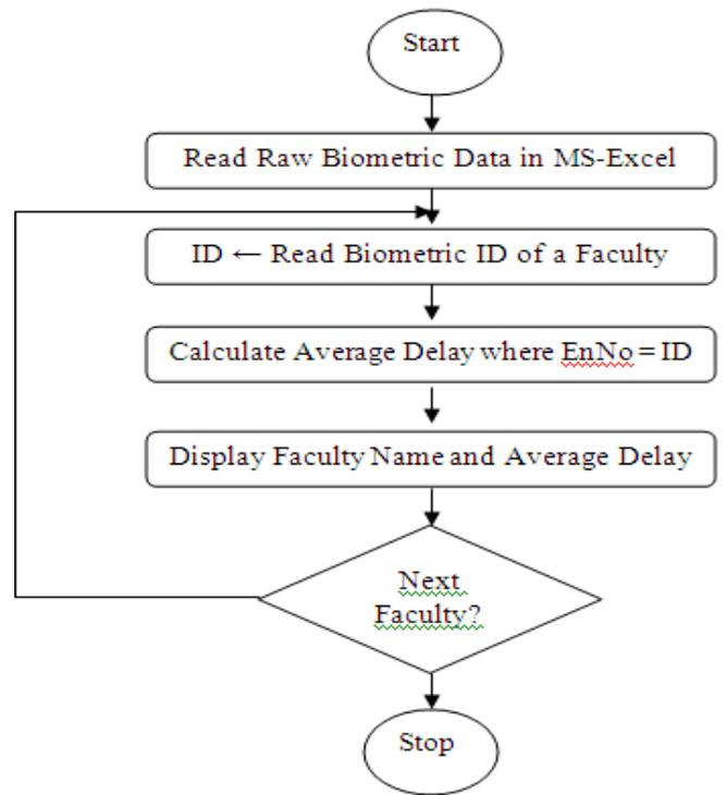
Figure 11(c). Control Flow Diagram for Computation of Faculty-wise Average Delay
