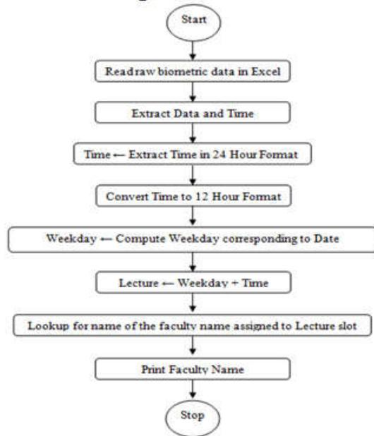
Figure 4(b). Control Flow Diagram for Computing Faculty column
