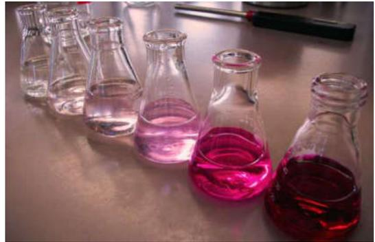
Fig. 2. Titration of citric acid using phenolphthalein produced by *Aspergillus niger*
