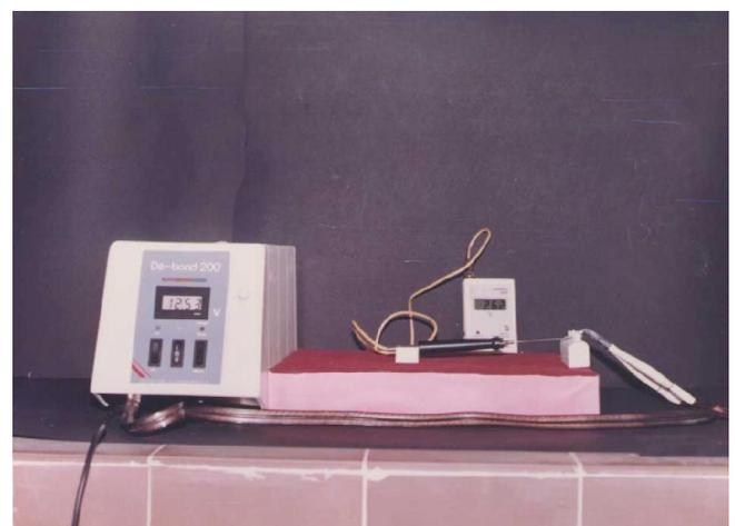
Fig. 2. ETD Machine with Pliers holding the bracket
