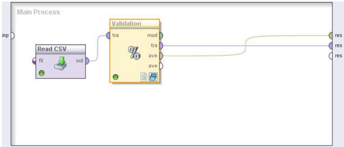
Fig. 2. The read CSV and cross validation operators of Rapidminer
