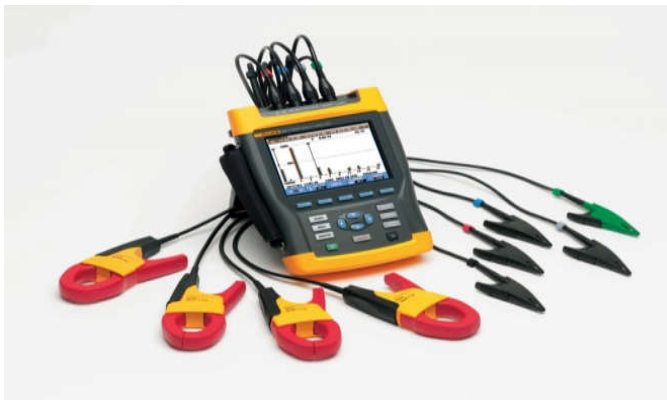
Fig. 6. Power Quality Analyzer Fluke 435
