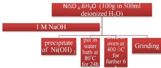
Figure 1. Schematic representation of co precipitation method of NiO nano composites
