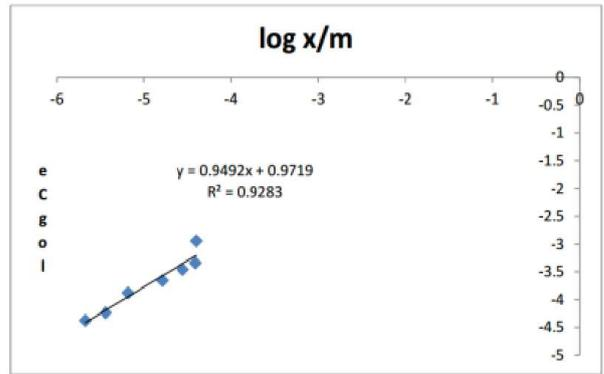
Figure 10. Optimization of Freundlich parameters at temperature 303K of NiO Nano particles
