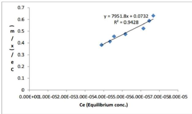
Figure 7. Optimization of Langmuir parameters at temperature 308K of NiO Nano particles
