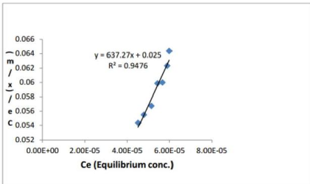
Figure 9. Optimization of Langmuir parameters at temperature 318K of NiO Nano particles
