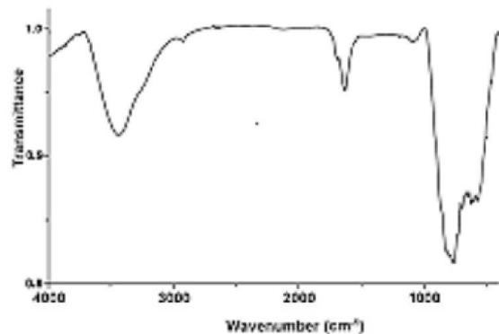
Figure 2. FTIR Spectrum of NiO nanoparticles
