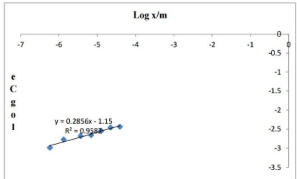
Figure 11. Optimization of Freundlich parameters at temperature 308K of NiO Nano particles
