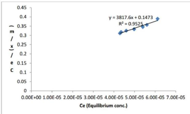
Figure 8. Optimization of Langmuir parameters at temperature 313K of NiO Nano particles
