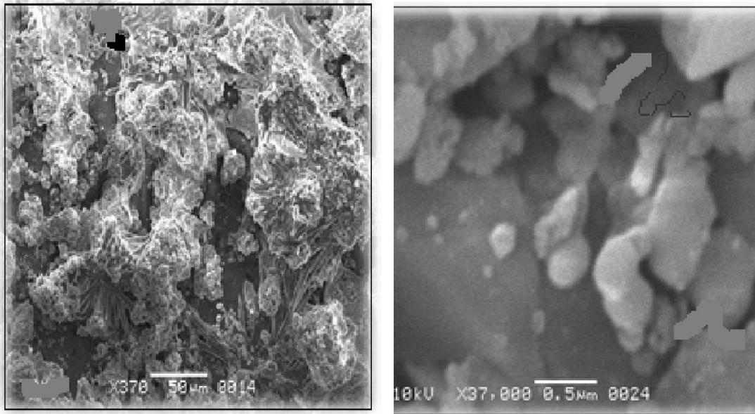
Figure 3. SEM image of NiO Nano composite before (size of nps are 58 micrometer) and after 91 Adsorption (size of nps are 0.5 micrometer)
