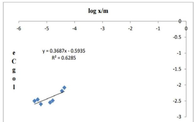
Figure 12. Optimization of Freundlich parameters at temperature 313K of NiO Nano particles
