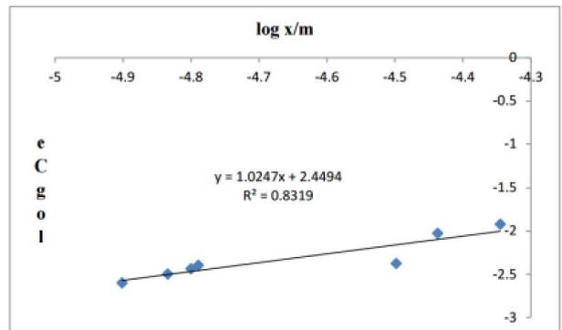
Figure 13. Optimization of Freundlich parameters at temperature 318K of NiO Nano particles
