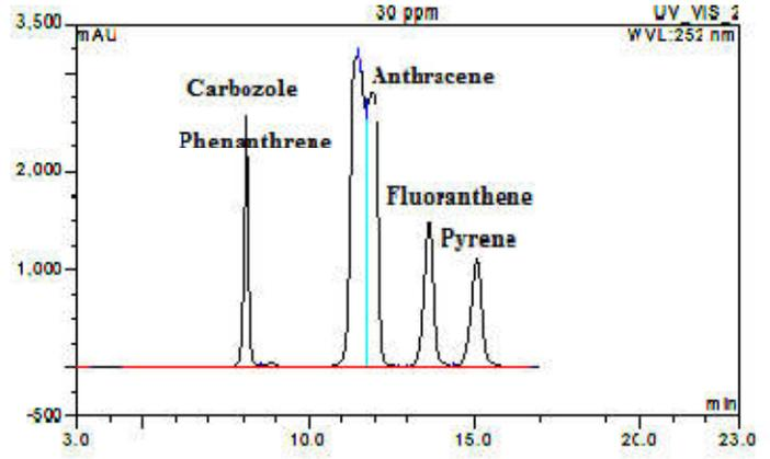
Figure 14. HPLC chromatogram for the four PAHs- Phenanthrene, Anthracene, Fluoranthene and Pyrene (Ashish *et al.*, 2016a) and carbazole at the concentrations of 30 and 20  $\text{mg}\cdot\text{dm}^{-3}$ , respectively
