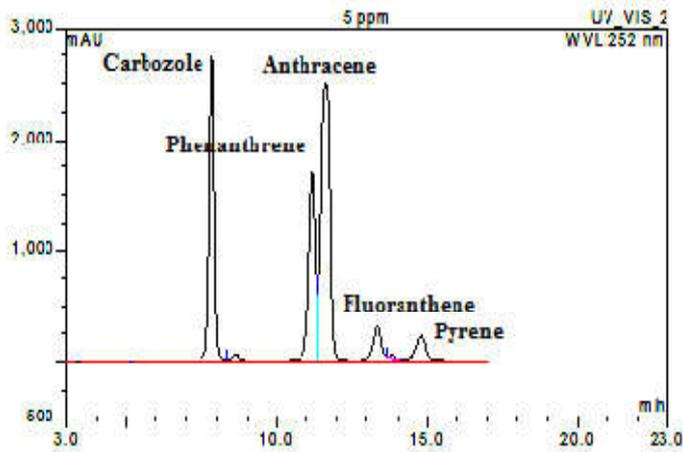
Figure 9. HPLC chromatogram for the four PAHs- Phenanthrene, Anthracene, Fluoranthene and Pyrene (Ashish *et al.*, 2016a) and carbazole at the concentrations of 5 and 20  $\text{mg}\cdot\text{dm}^{-3}$ , respectively
