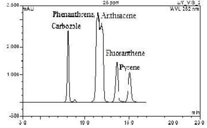
Figure 13. HPLC chromatogram for the four PAHs- Phenanthrene, Anthracene, Fluoranthene and Pyrene (Ashish *et al.*, 2016a) and carbazole at the concentrations of 25 and 20  $\text{mg}\cdot\text{dm}^{-3}$ , respectively
