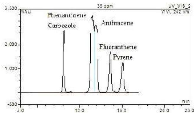
Figure 15 - HPLC chromatogram for the four PAHs- Phenanthrene, Anthracene, Fluoranthene and Pyrene (Ashish *et al.*, 2016a) and carbazole at the concentrations of 35 and 20 mg.dm<sup>-3</sup>, respectively
