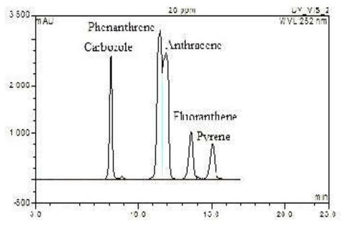
Figure 12. HPLC chromatogram for the four PAHs- Phenanthrene, Anthracene, Fluoranthene and Pyrene (Ashish *et al.*, 2016a) and carbazole at the concentrations of 20 and 20  $\text{mg}\cdot\text{dm}^{-3}$ , respectively
