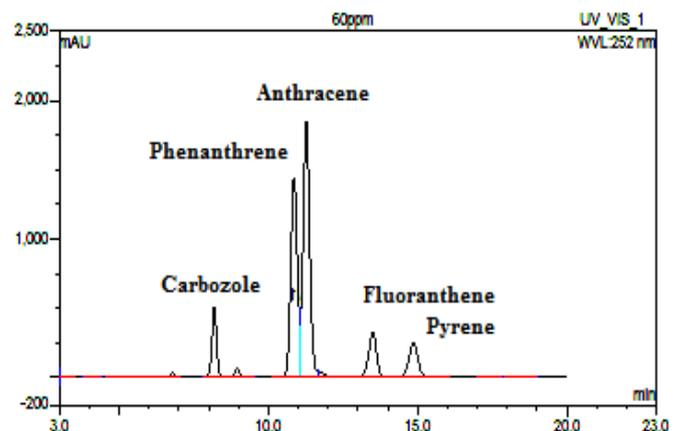
Figure 4. HPLC chromatogram for the four PAHs-Phenanthrene, Anthracene, Fluoranthene and Pyrene (Ashish *et al.*, 2016a) and carbozole at the concentrations of 60 and 45 mg.dm<sup>-3</sup>, respectively
