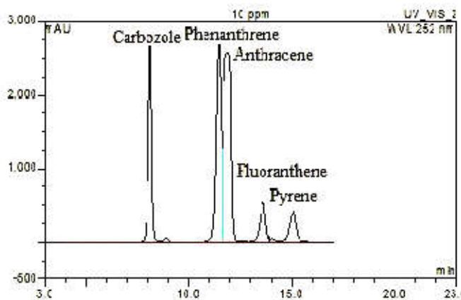
Figure 10. HPLC chromatogram for four PAHs- Phenanthrene, Anthracene, Fluoranthene and Pyrene (Ashish *et al.*, 2016a) and carbazole at the concentrations of 10 and 20  $\text{mg}\cdot\text{dm}^{-3}$ , respectively
