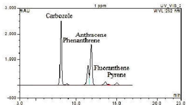
**Figure 8. HPLC chromatogram for the four PAHs-Phenanthrene, Anthracene, Fluoranthene and Pyrene (Ashish *et al.*, 2016a) and carbozole at the concentrations of 1 and 20 mg.dm<sup>-3</sup>, respectively**
