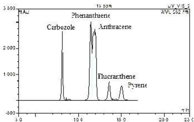
Figure 11. HPLC chromatogram for the four PAHs- Phenanthrene, Anthracene, Fluoranthene and Pyrene (Ashish *et al.*, 2016a) and carbazole at the concentrations of 15 and 20  $\text{mg}\cdot\text{dm}^{-3}$ , respectively
