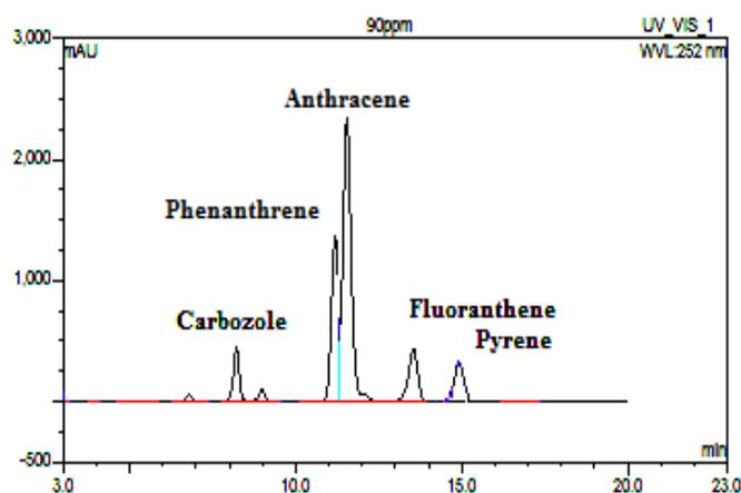
Figure 6. HPLC chromatogram for the four PAHs- Phenanthrene, Anthracene, Fluoranthene and Pyrene (Ashish *et al.*, 2016a) and Carbozole at the concentrations of 90 and 45 mg.dm<sup>-3</sup>, respectively
