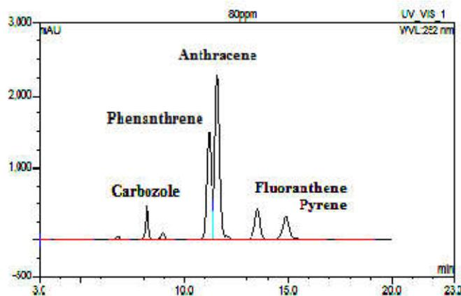
Figure 5. HPLC chromatogram for the four PAHs- Phenanthrene, Anthracene, Fluoranthene and Pyrene (Ashish *et al.*, 2016a) and Carbozole at the concentrations of 80 and 45 mg.dm<sup>-3</sup>, respectively
