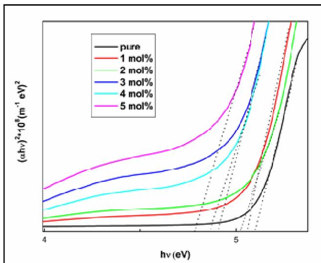
Fig. 6.  $(\alpha hv)^2$  vs  $h\nu$  plots of pure and  $Fe^{3+}$  doped MAA:EA copolymer electrolytes
