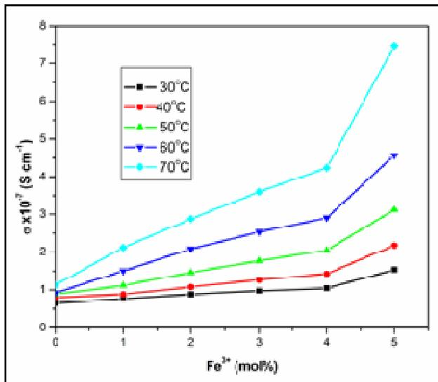
Fig.2. Conductivity vs. dopant concentration plots of (MAA:EA/ $\text{Fe}^{3+}$ ) copolymer electrolyte system at different temperatures
