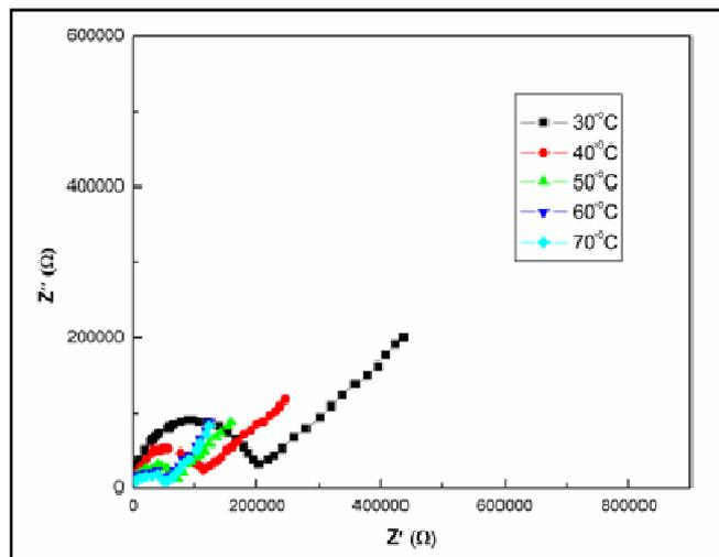
Fig.1. Cole–Cole plots for (MAA:EA/Fe<sup>3+</sup>) (5mol%) copolymer electrolyte at different temperatures
