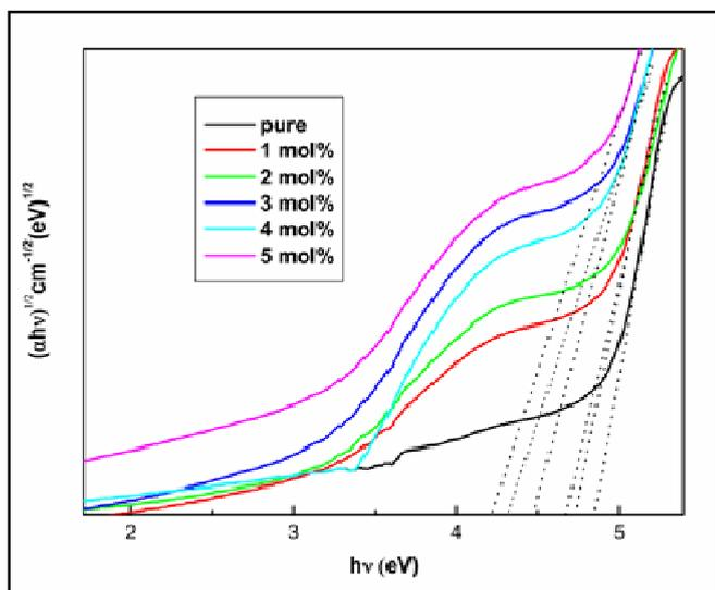
Fig. 7.  $(\alpha hv)^{1/2}$  vs  $h\nu$  plots of pure and  $Fe^{3+}$  doped MAA:EA copolymer electrolytes
