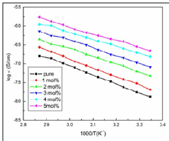
Fig.3. Inverse temperature dependent conductivity of pure MAA:EA and  $\text{Fe}^{3+}$  doped copolymer electrolyte films of different concentration
