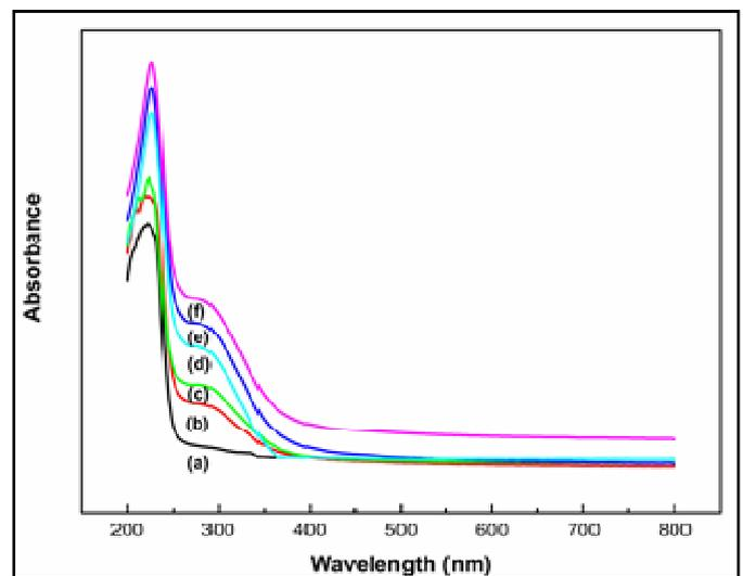
**Fig. 4. Ultra Violet absorption spectra for MAA:EA copolymer electrolytes containing Fe<sup>3+</sup> (a) pure (b) 1 mol% (c) 2 mol% (d) 3 mol%. (e) 4 mol% (f) 5 mol%**
