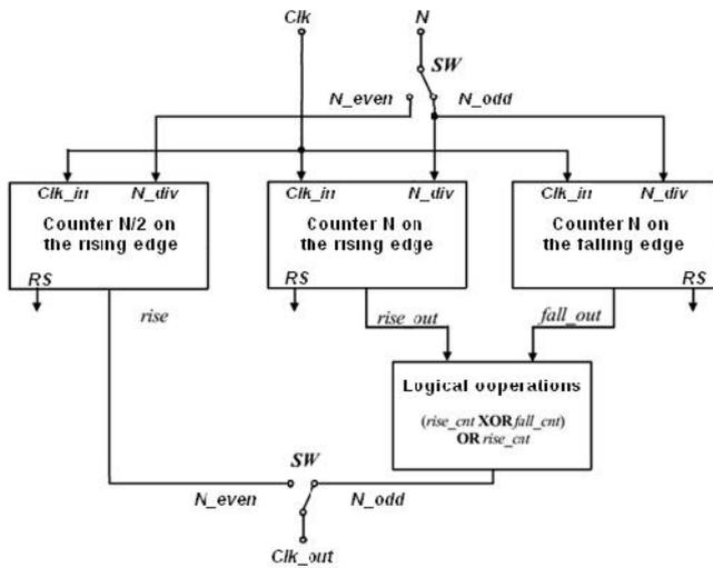
Figure 4. Proposed Architecture for the frequency divider
