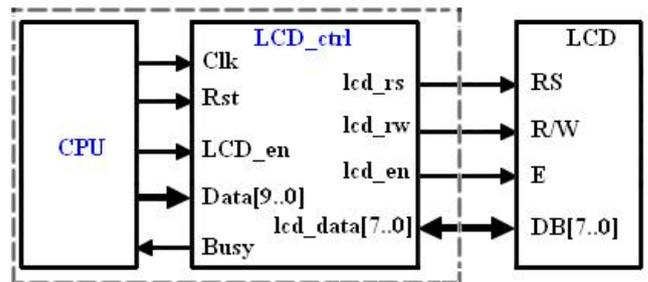
**Figure 10. Controller LCD module**
