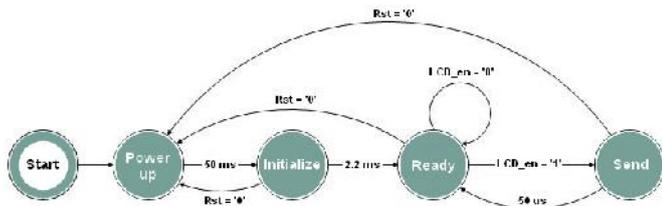
Figure 11. State machine for managing the LCD
