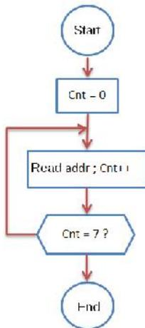
**Figure 8. Reading flowchart of the program memory**
