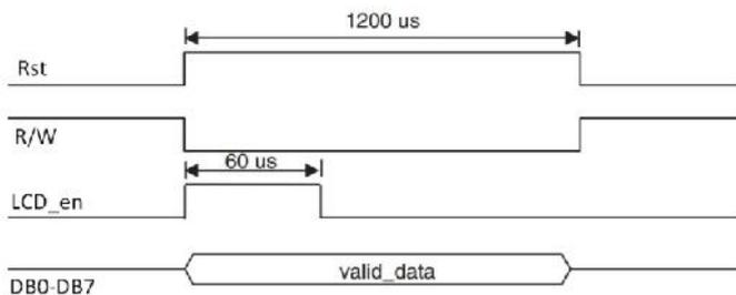
Figure 12. Write timing diagram for the LCD
