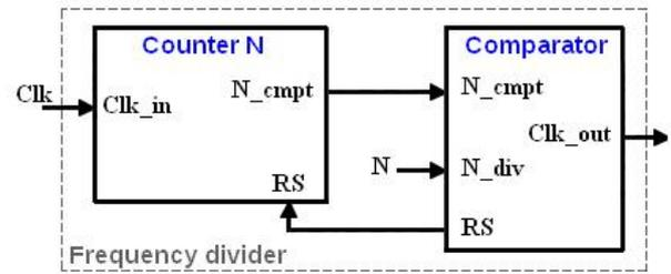
Figure 3. Block diagram of the frequency divider
