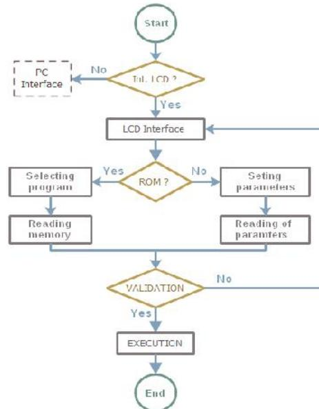
Figure 13. Process operation of the user interface
