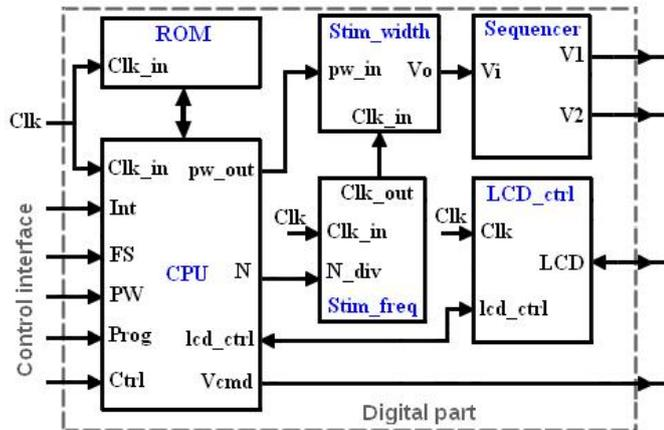
Figure 2. Proposed architecture for the digital part
