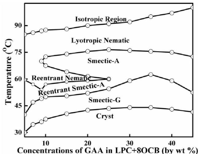
Figure 1. Partial phase diagram for the mixture of GAA in LPC+8OCB
