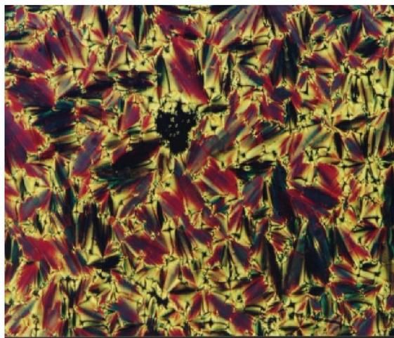
b). Focal conic fan texture of Smectic-A phase (250X).
