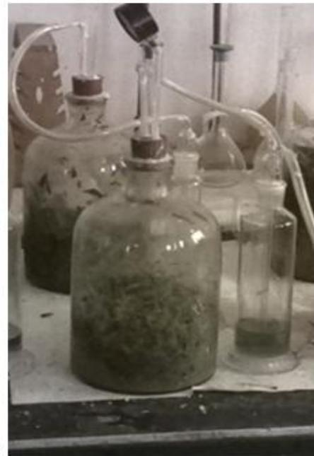
Figure 1. Single Biomethanation unit (Digester)
