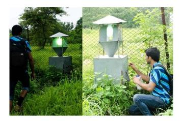
Figure A personal funnel shaped mercury light trap
