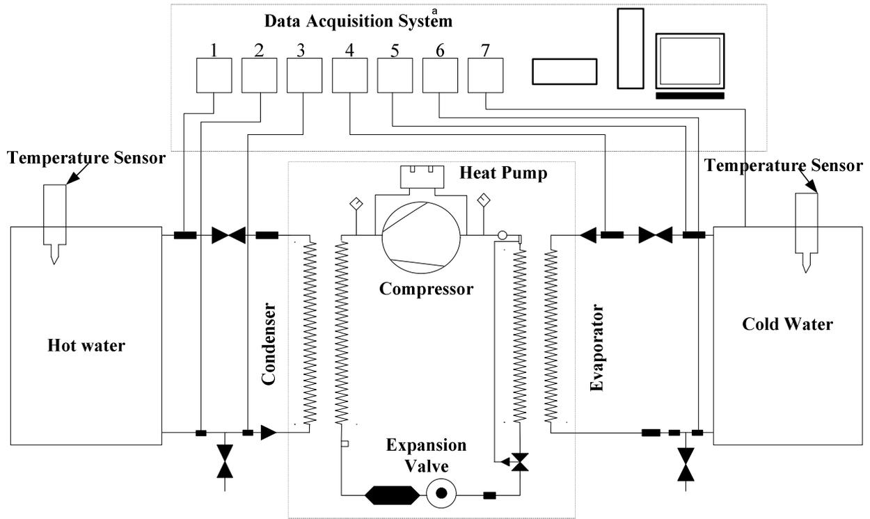
Fig. 4. Heat pump monitoring system
