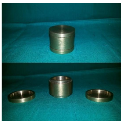
Fig. 1. Customised brass metal cylindrical mold
