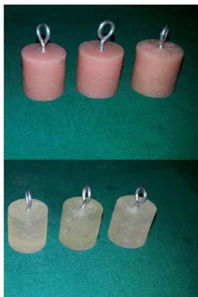
Fig. 2. Fabricated sample pairs with attached metal hook
