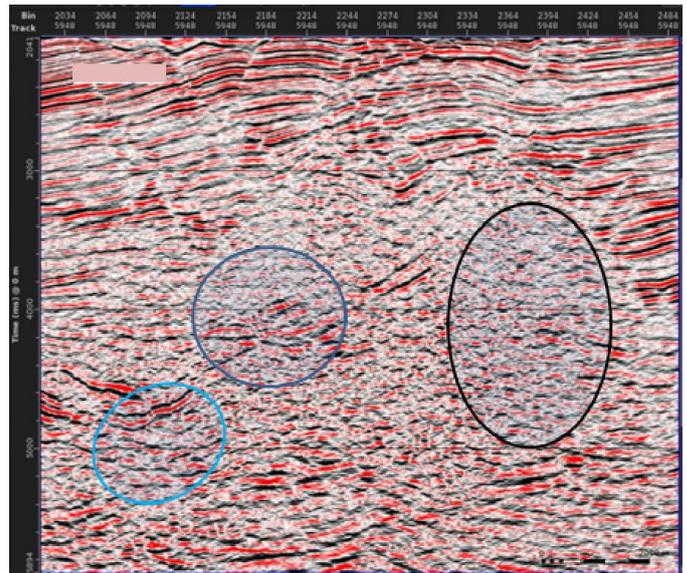
Fig. 4. 3d PSDM section Prior to Detailed velocity analysis as applied in this study; beyond 3000ms, reflection events are indiscernible, fault lines and structures are unidentifiable
