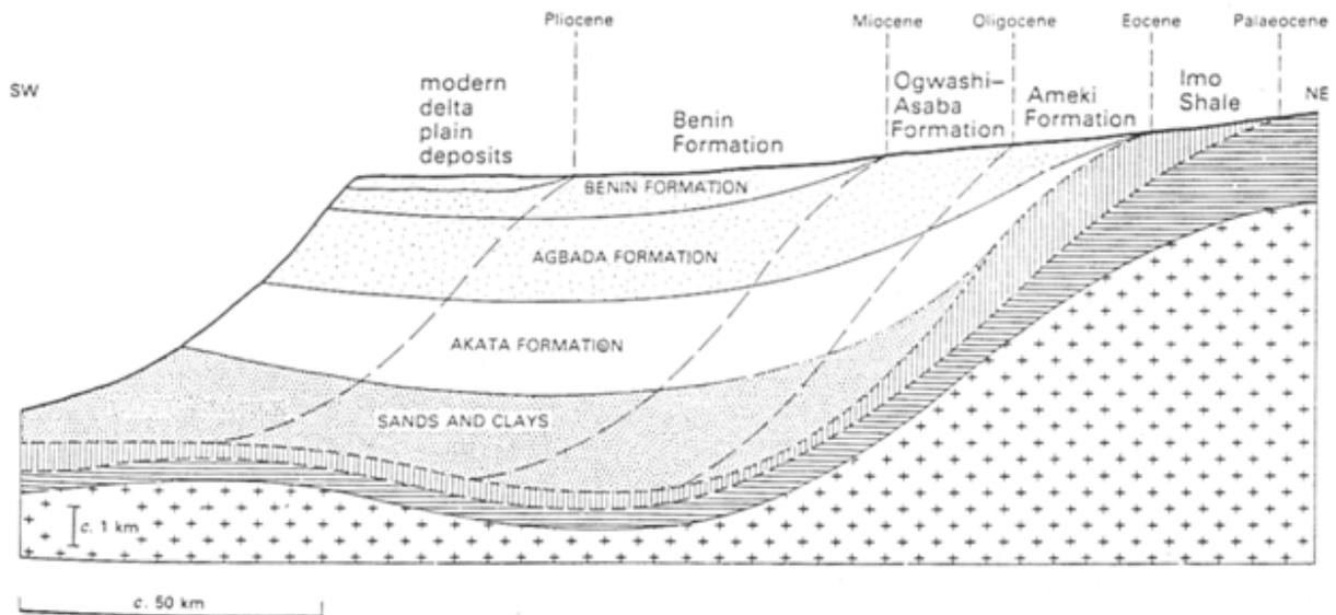
Fig. 2. Longitudinal Cross section showing the successive Formations in the Niger Delta
