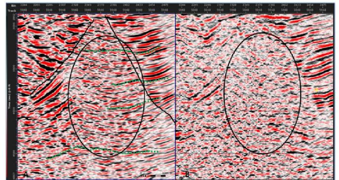
Fig. 6. Comparison of areas at the footwall of the fault; Observe the chaotic nature of reflection events within the circled zone in B; Events are more continuous in the corresponding circle in A – (illustrated by the green dotted lines in A)
