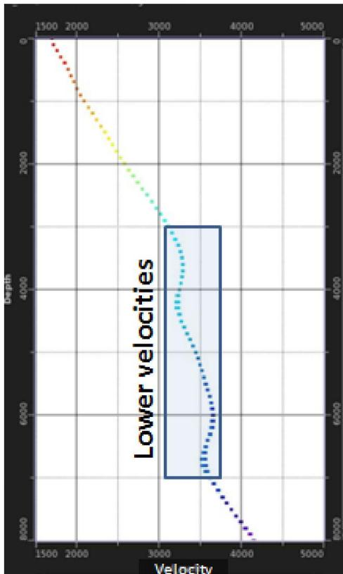
Fig. 3. Velocity-Depth Plot showing prevalence of low velocities at depth
