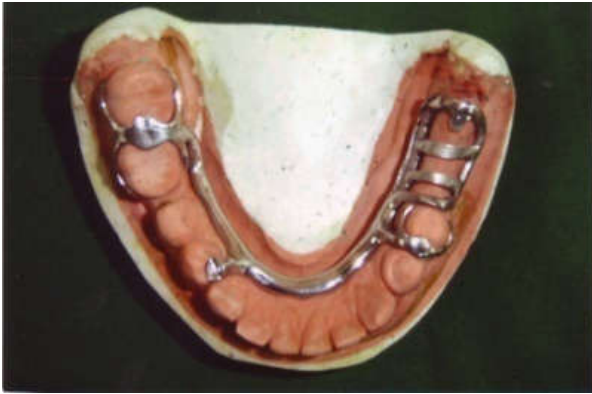
Fig.1. Cast partial denture metal framework
