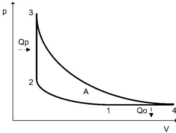
$$\eta_H = 1 - \gamma \frac{T_2}{T_3} \left( \frac{T_4}{T_3} \right)^{\frac{\gamma}{\gamma-1}} - 1$$
