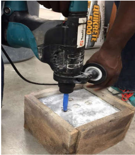
Fig. 4. Collection of powder concrete samples
