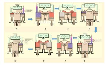
Figure 2. Working cycle of 5 stroke engine Source: Schmitz, 2003
