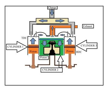
Figure 1. Five stroke engine with three cylinders Source: Schmitz, 2003
