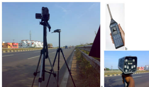
Fig (2) a. A typical measurement location, b. Norsonic sound level meter and c. Hand held radar gun.
