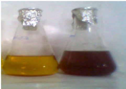
Fig 1. Formation of silver nanoparticles a – Leaf extract, b – Leaf extract + AgNO 3 after 48 hours
