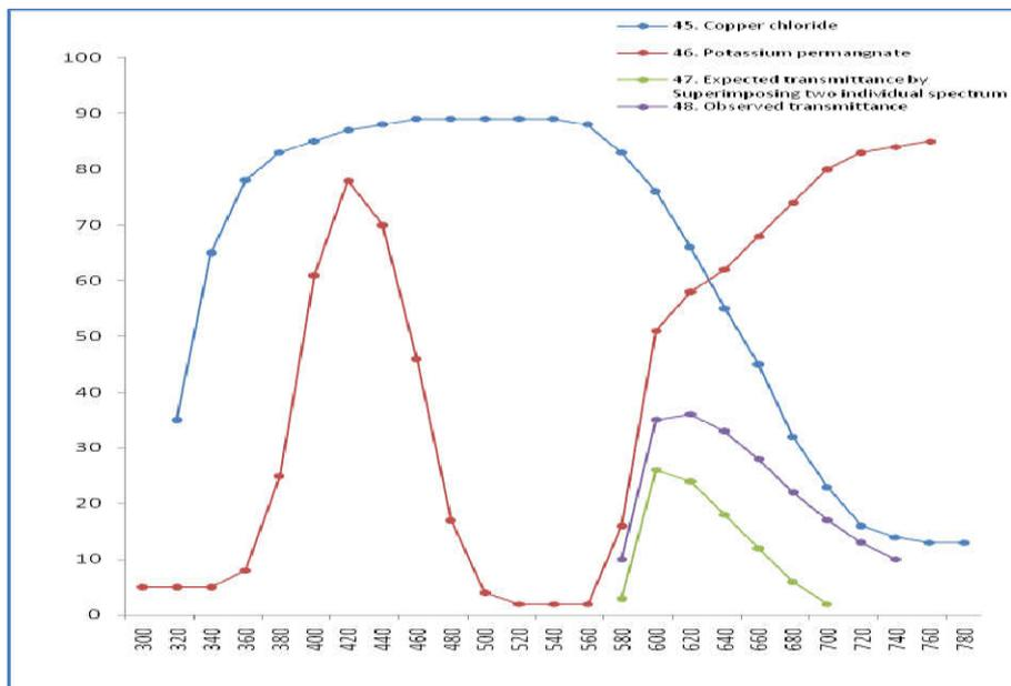
Fig. 4. Individual, expected and observed percentage transmittance of Copper chloride and Potassium permanganate at various wavelength
