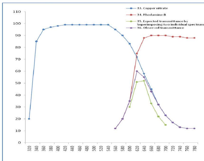
**Fig. 2. Individual, expected and observed percentage transmittance of Copper nitrate and Rhodamine-B at various wavelength**
