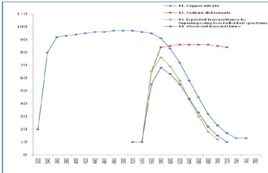
Fig. 3. Individual, expected and observed percentage transmittance of Copper nitrate and Sodium dichromate at various wavelength
