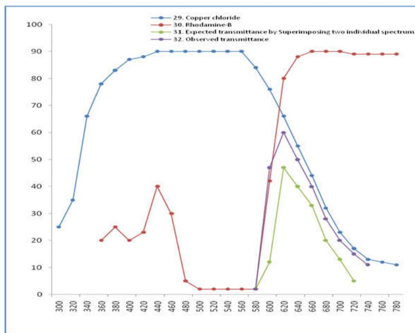
**Fig. 1. Individual, expected and observed percentage transmittance of Copper chloride and Rhodamine-B at various wavelength**
