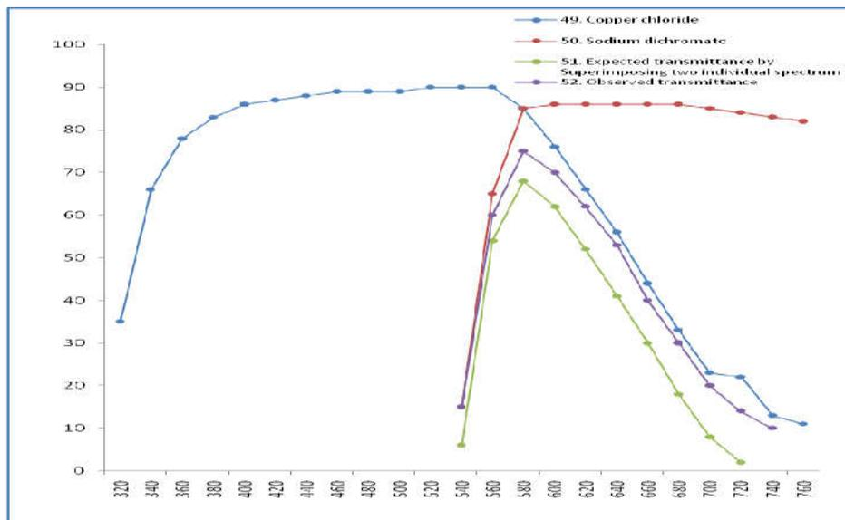
Fig. 5. Individual, expected and observed percentage transmittance of Copper chloride and Sodium dichromate at various wavelength
