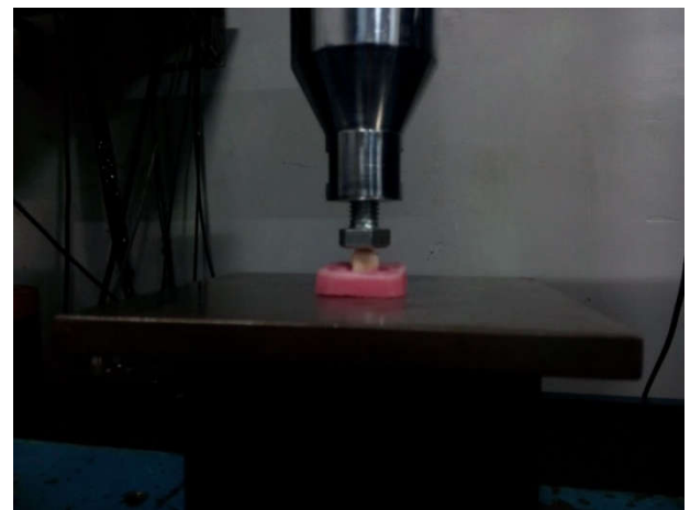
Figure No. 2. Sample under Universal Testing Machine
