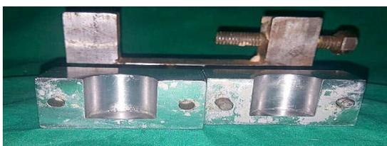
A stainless steel split mould of cylindrical shape was fabricated with diameter 25 mm and height 25 mm for surface hardness
