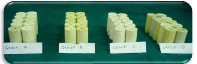
**Samples for testing compressive strength**
