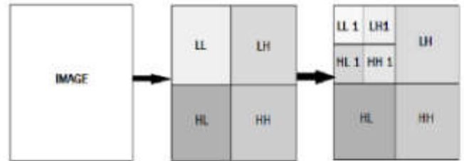
Fig.2. Frequency sub band second level decomposition of an image (Asna Furqan and Munish Kumar, 2015)
