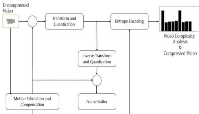
Fig. 3. Architecture of Video Compression
