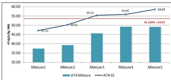
**Figure 5. The AT<sub>4</sub> values of the sewage sludge in the mixture considering sawdust and mixture AT<sub>4</sub> by mixing ratio**
