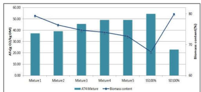
Figure 4. AT<sub>4</sub> values and biomass content according to mixing ratio
