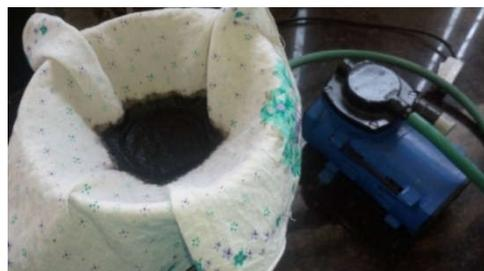
Fig.5. Washing of carbonized powder
