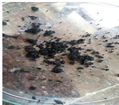
Fig.6. Final Activated Carbon of Stems Water Hyacinth
