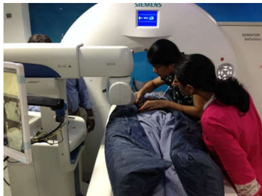
Fig. 1. Immobilisation bed and robotic biopsy system used for positioning of patient
