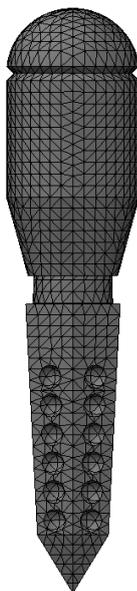
Figure 19. IHPP Implant Configuration 2 test with support – Mesh of the mathematical model with tetrahedral elements
