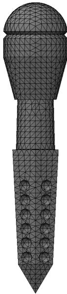
Figure 18. IHPP Implant Configuration 1 test with support – Mesh of the mathematical model with tetrahedral elements
