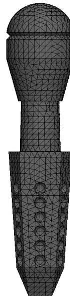
Figure 21. IHPP Implant Configuration 4 test with support – Mesh of the mathematical model with tetrahedral elements.
