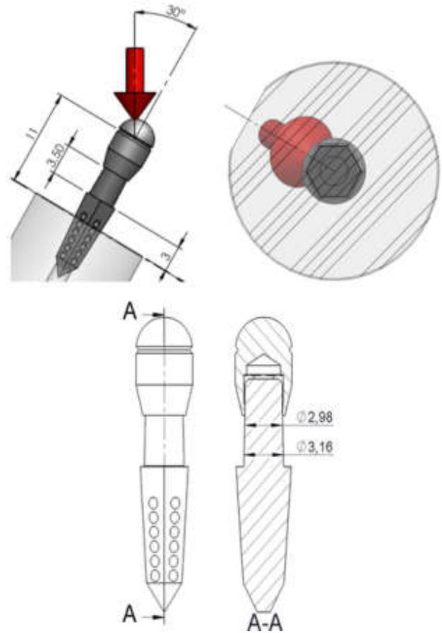
Figure 28. RHPP Implant Configuration 5 test with support – Main dimensions for the structural analysis (Dimensions in millimeters)
