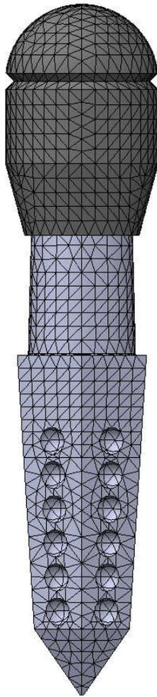
Figure 22. RHPP Implant Configuration 5 test with support – Mesh of the mathematical model with tetrahedral elements
