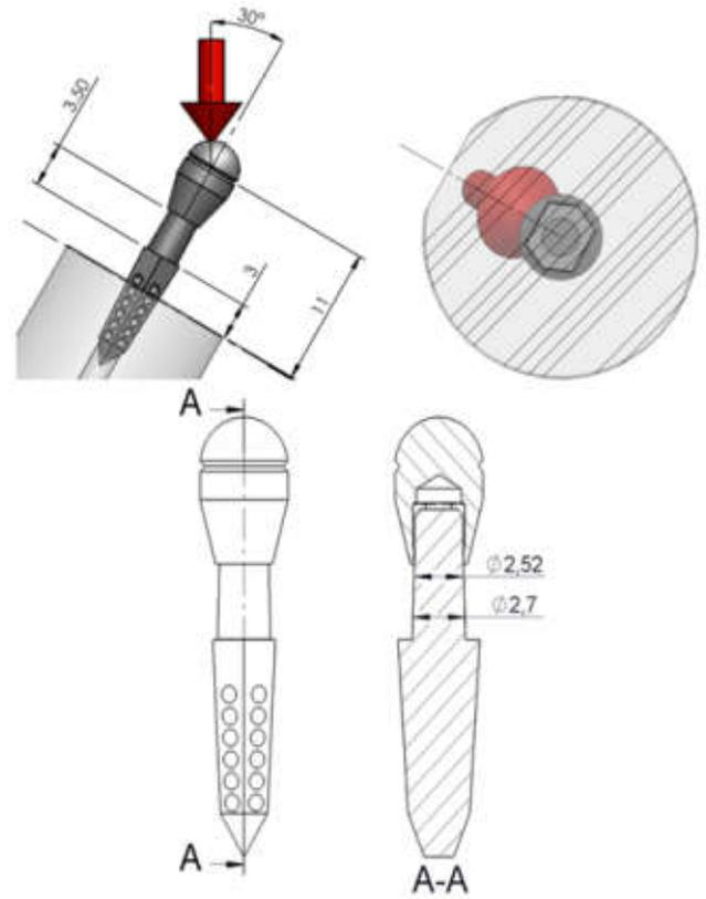
Figure 24. IHPP Implant Configuration 1 test with support – Main dimensions for the structural analysis (Dimensions in millimeters)
