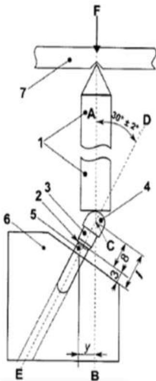
Figure 23. Test scheme indicated by the UNI EN ISO 14801:2017
