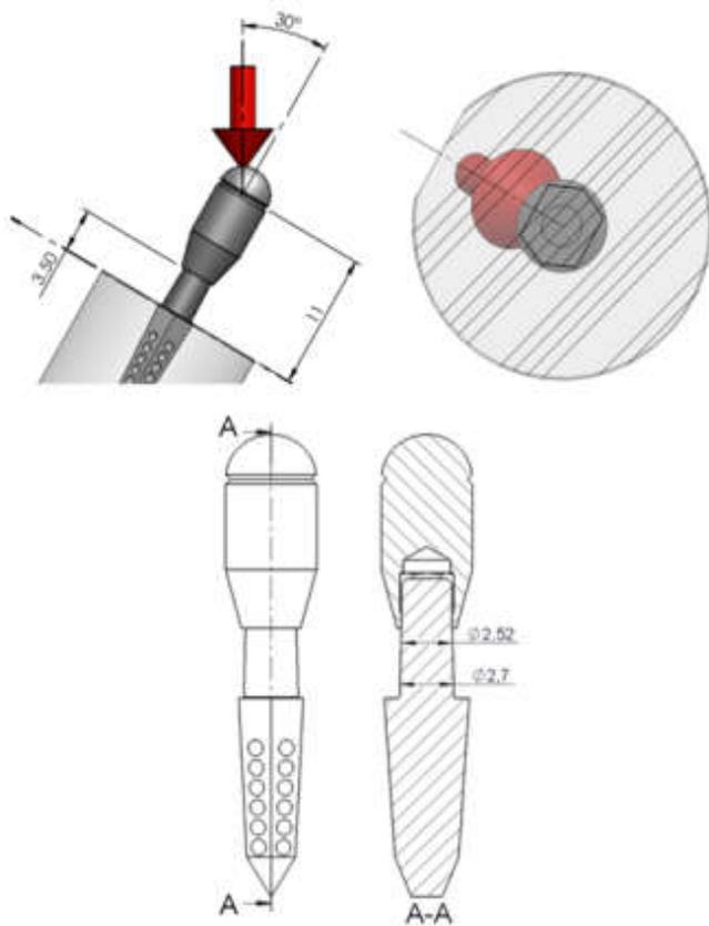
Figure 26. IHPP Implant Configuration 3 test with support – Main dimensions for the structural analysis (Dimensions in millimeters)
