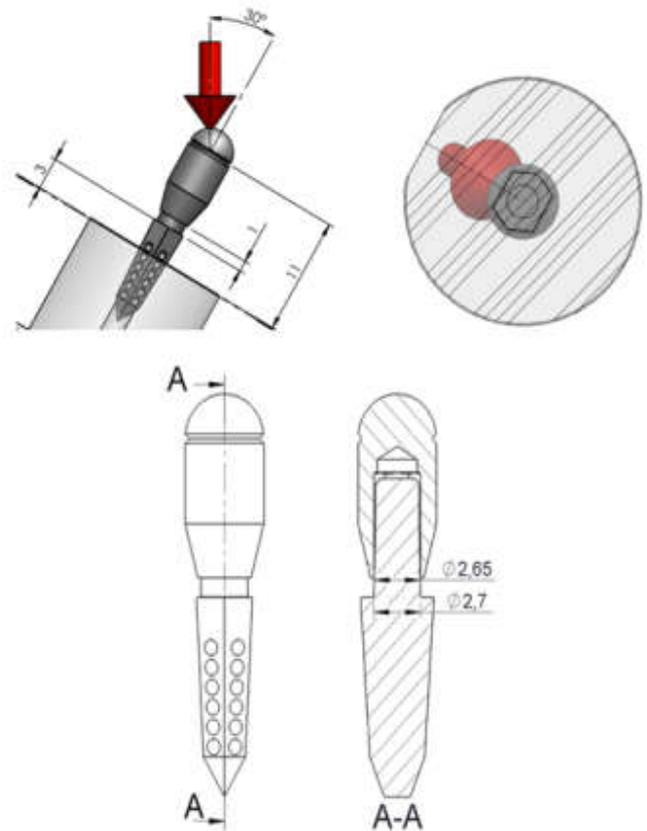
Figure 25. IHPP Implant Configuration 2 test with support – Main dimensions for the structural analysis (Dimensions in millimeters)
