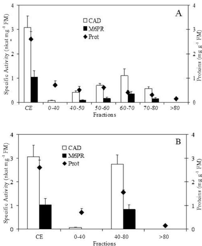
**Figure 5. Precipitation and fractionation with the ammonium sulphate. A- activities and proteins in the fractions from 0 to 100%; B- activities and proteins in the combined fraction 40-80%. FM: fresh matter; CE: crude extract. (25 and 100 $\mu$ g of proteins are used for the analysis SDS-PAGE and the measurement of the enzymatic activities respectively).**
